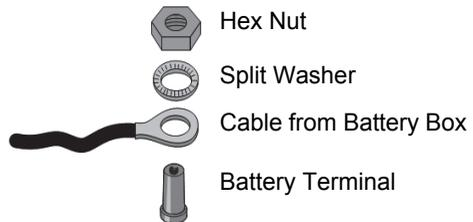
**Figure 3-3** Preparing the Battery Bank
