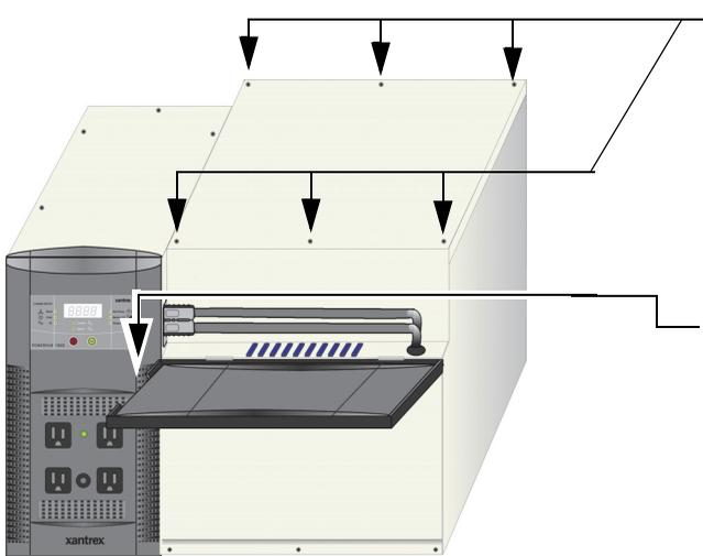
2. Align the screw holes from the top to the enclosure.
