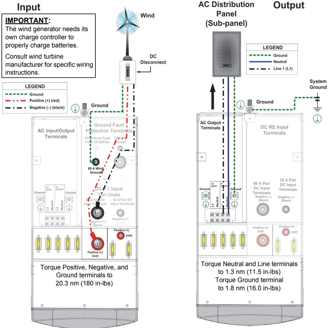
**Figure 3-16** Connecting the DC Input (Renewable Energy Wind)
