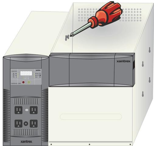
**Important:** Attaching the battery box(es) to the inverter grounds the chassis' of the two components and is required, not optional.
