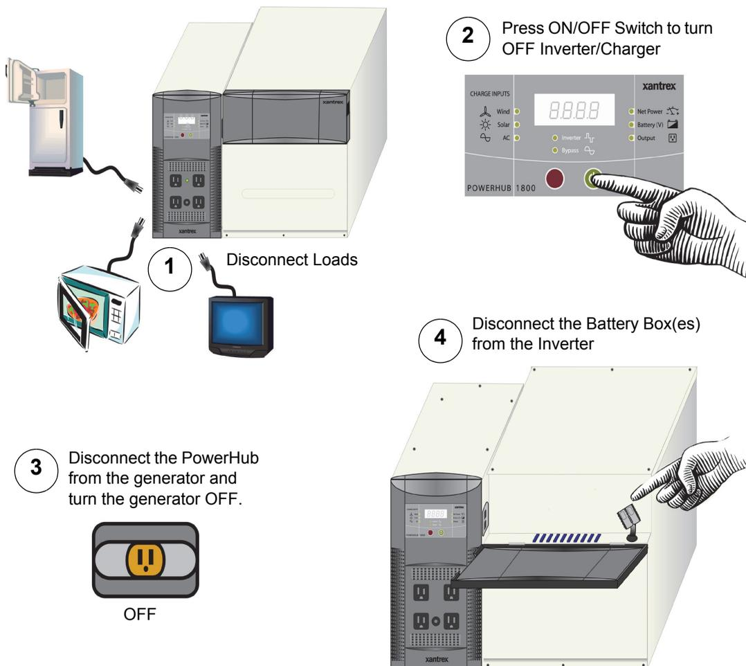
**Figure ii** Power Down Procedure for Softwired Installations
