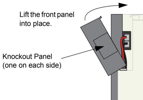
Gently push the lip on the front panel under the lip on the top of the battery box enclosure.
