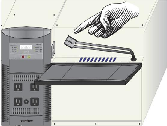
**1** Connect the Battery Box(es) to the Inverter.
