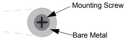
2. Loosen these screws just enough to allow the keyhole slots on the side of the battery Box to slip over the top of them. Do NOT remove these screws completely.
