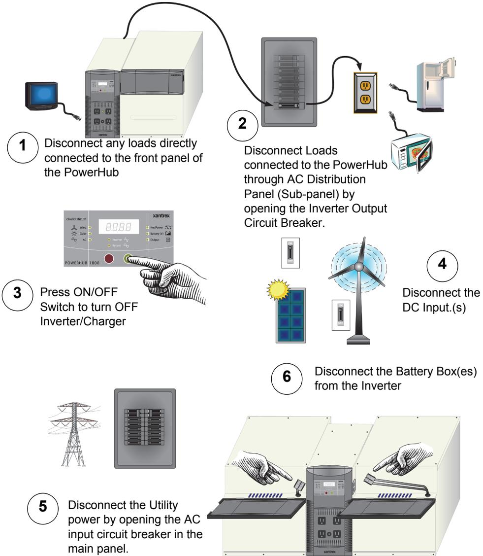
**Figure iii** Power Down Procedure for Hardwired Installations
