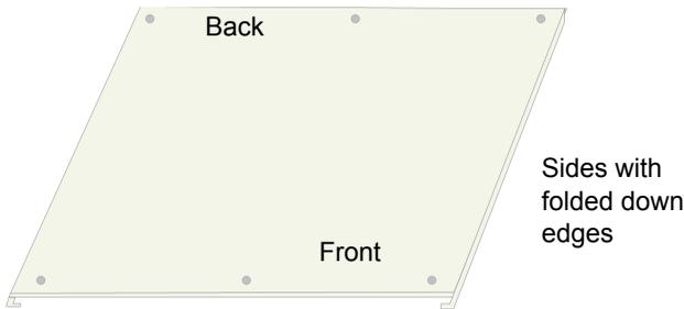
1. Place the top to the battery box on the enclosure, back edge first so that the back edge of the enclosure is inserted into the folded down edges of the sides of the top.
