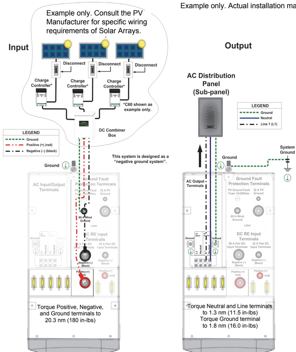
Figure 3-15 Connecting the DC Input (Renewable Energy Solar Array)
