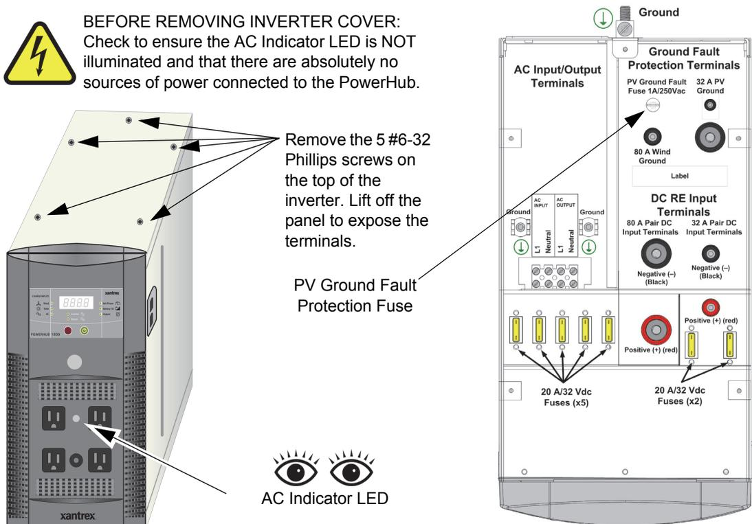
**Figure 3-22** Replacing Ground Fault Protection Fuse
