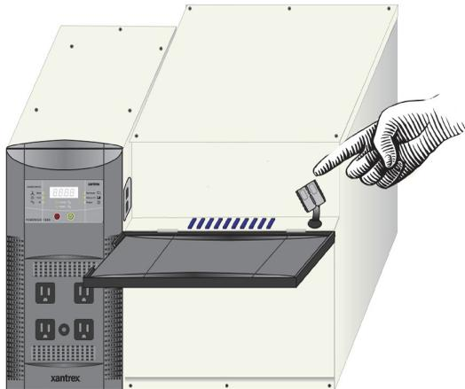
**Figure 3-20** Power Down Procedure for Softwired Installations
