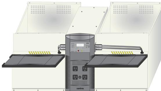
**Figure 3-6** Connecting Two Battery Boxes to the Inverter
