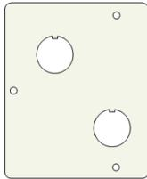
3. Locate the AC Accessory Plate and remove one or the two of the knockouts depending on whether both input and output wiring will be needed. If only input is needed, then only remove one knockout.
