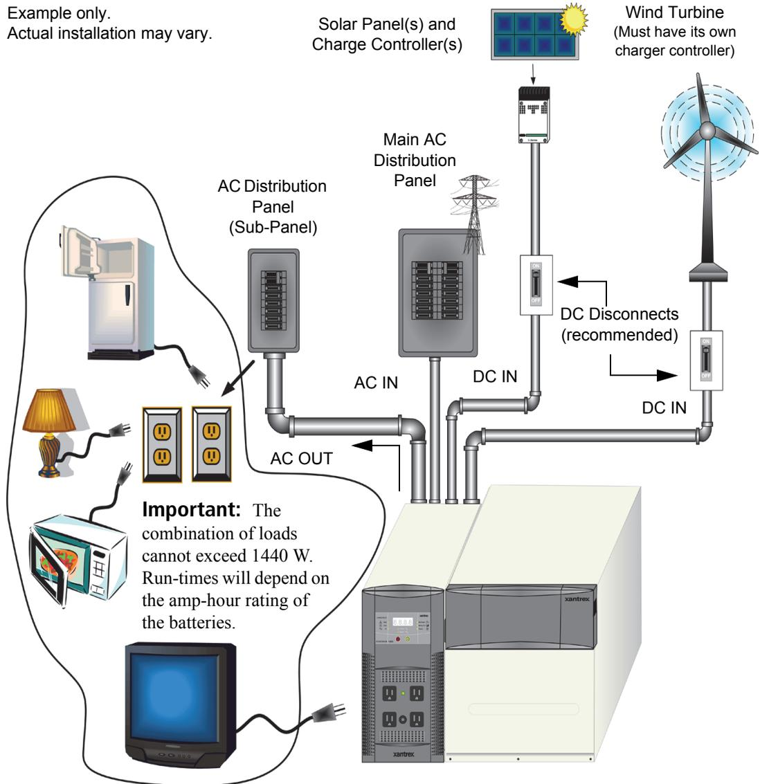
**Figure 1-8** Hardwired Combination Applications
