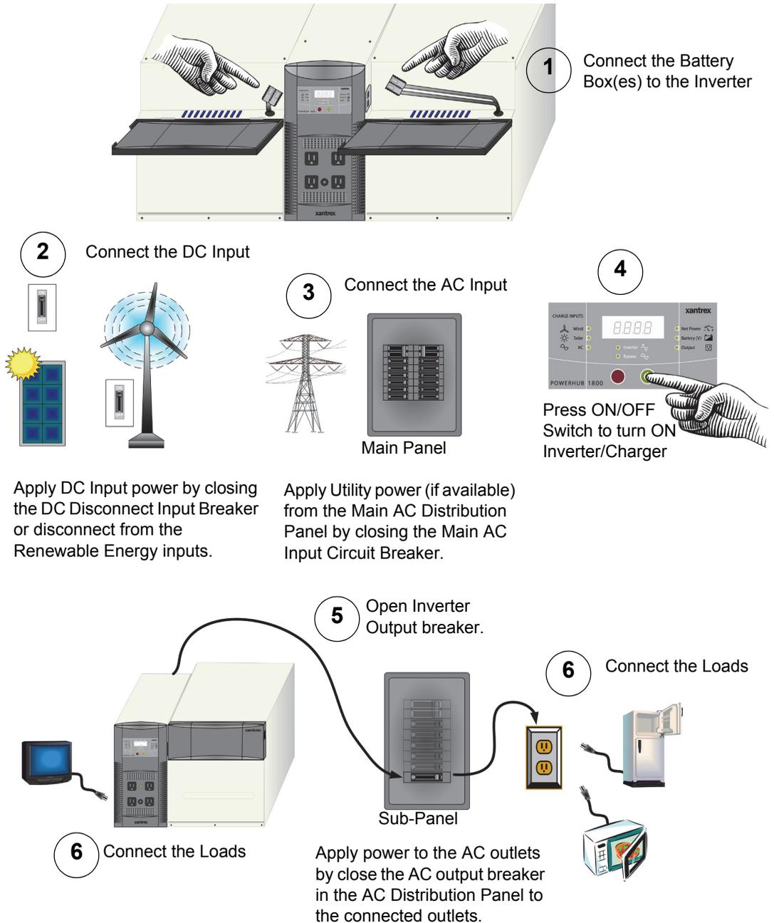
**Figure 3-19** Power Up Procedure for Hardwired Installations
