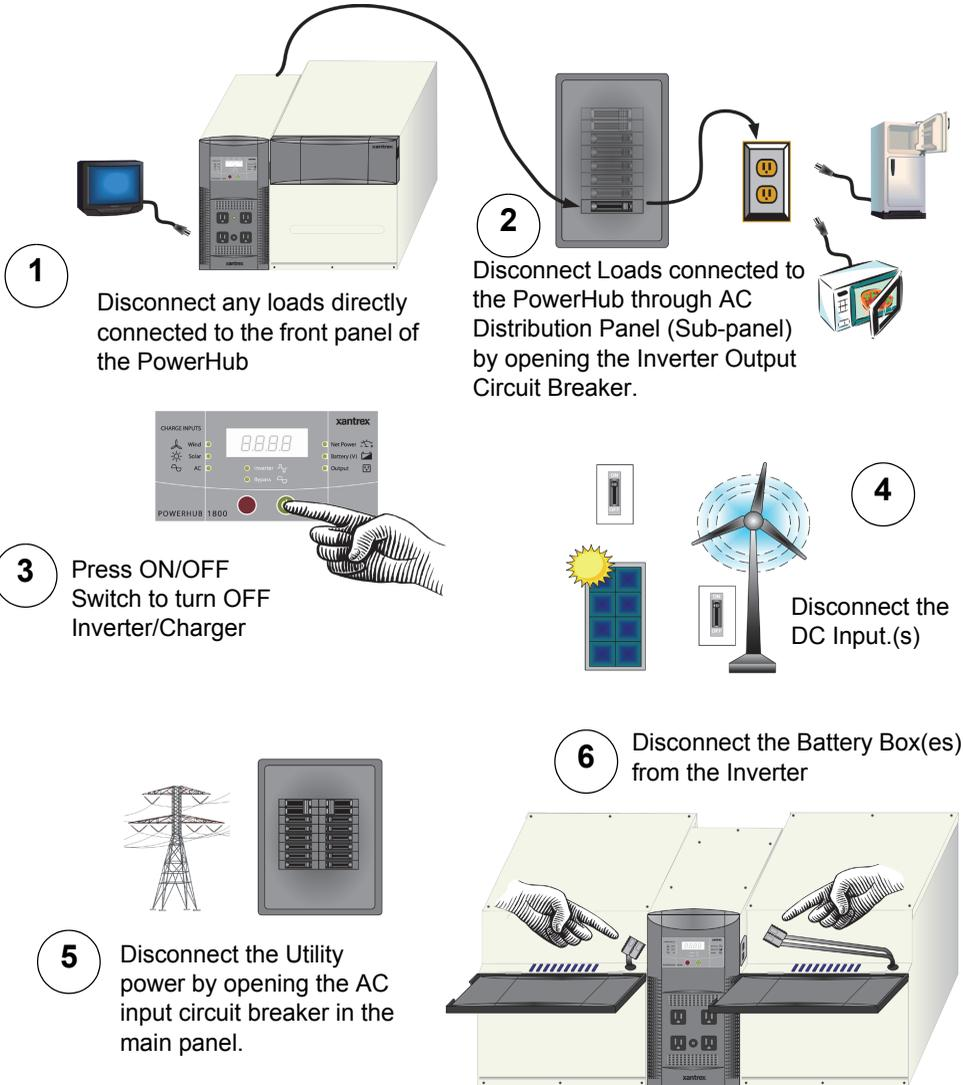
**Figure 3-21** Power Down Procedure for Hardwired Installations
