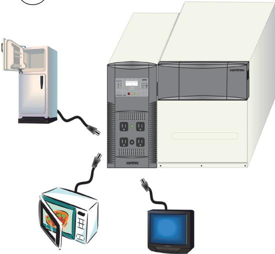
**2** Press ON/OFF Switch to turn OFF Inverter/Charger.
