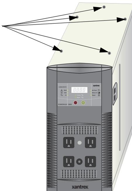
Figure 3-17 Replacing the Top Cover on the Inverter
