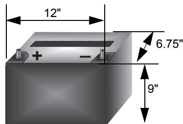
Figure 2-2 Battery Box and Battery Size
