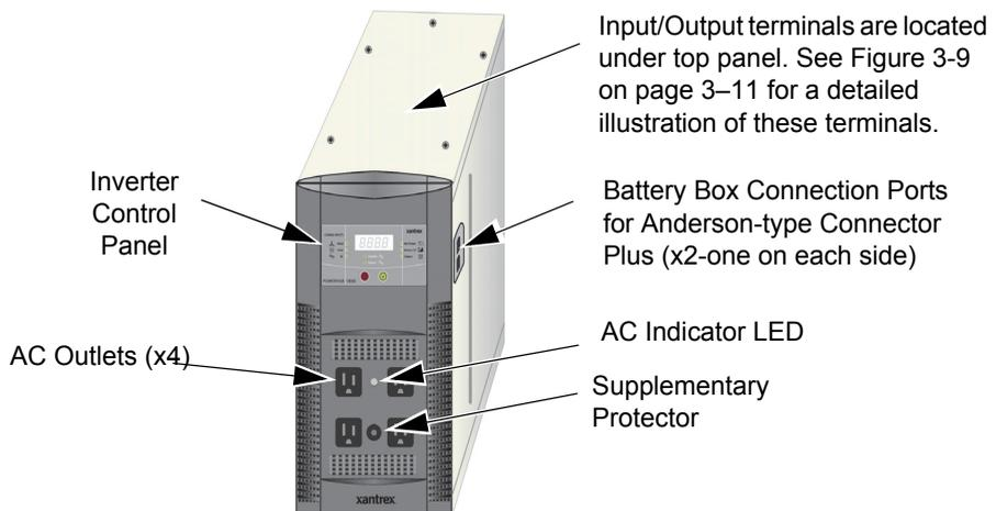
**Figure 1-3** PowerHub 1800 Features
