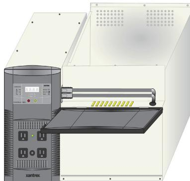
**Figure 3-5** Connecting the Battery Bank to the Inverter
