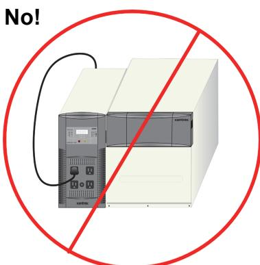
Do not plug input cord into output socket.
