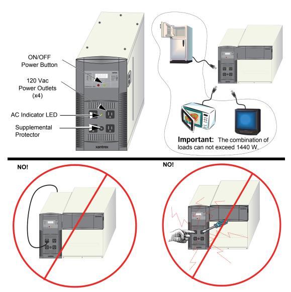
Figure 2-6 Connecting AC Loads
