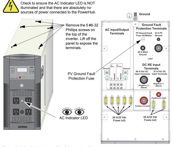
**Figure 3-1** Replacing Ground Fault Protection Fuse
