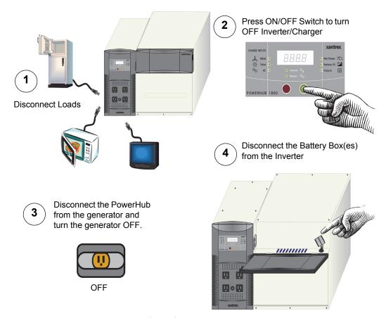
Figure ii Power Down Procedure for Softwired Installations
