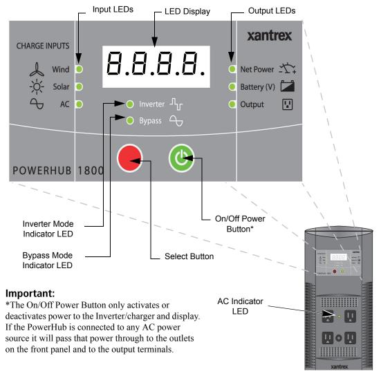
Figure 2-1 The PowerHub 1800 Inverter Control Panel
