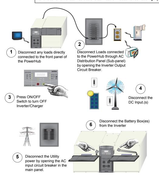
Figure iii Power Down Procedure for Hardwired Installations
