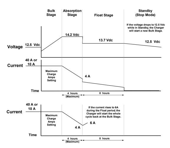
Figure A-1 Three-Stage Charging Process
