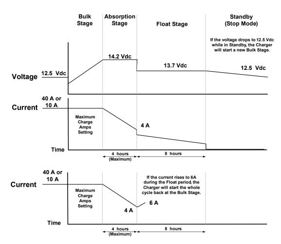
**Figure 1-3** Three-Stage Charging Process
